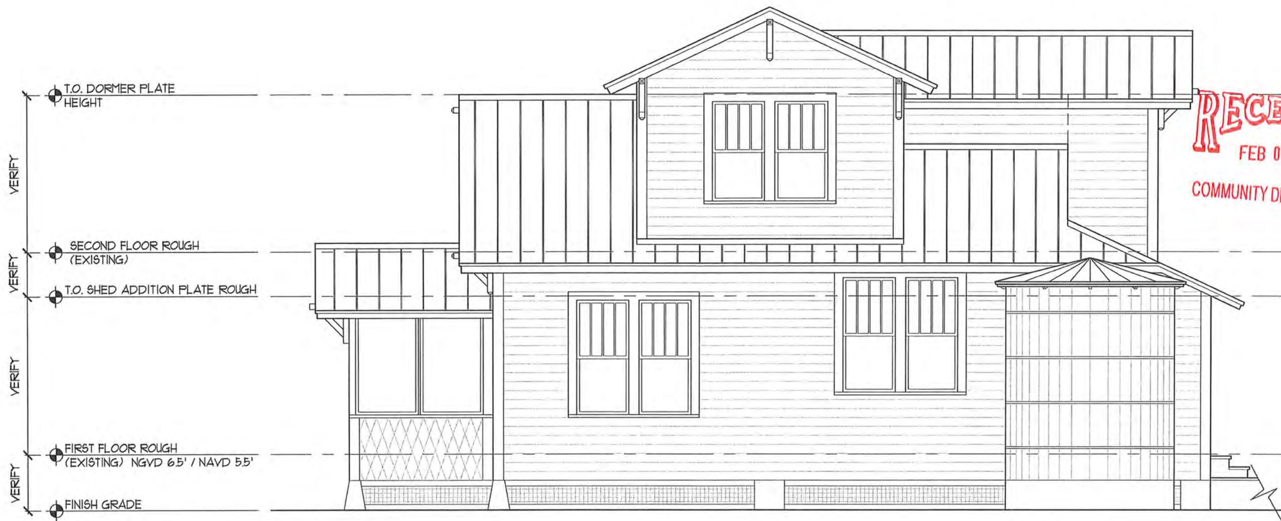
As-Built South Elevation
