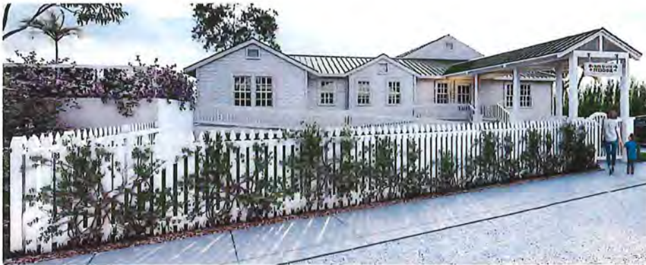
5-ft high picket fence along the Palm Ave property line turning west to the concrete fence.
