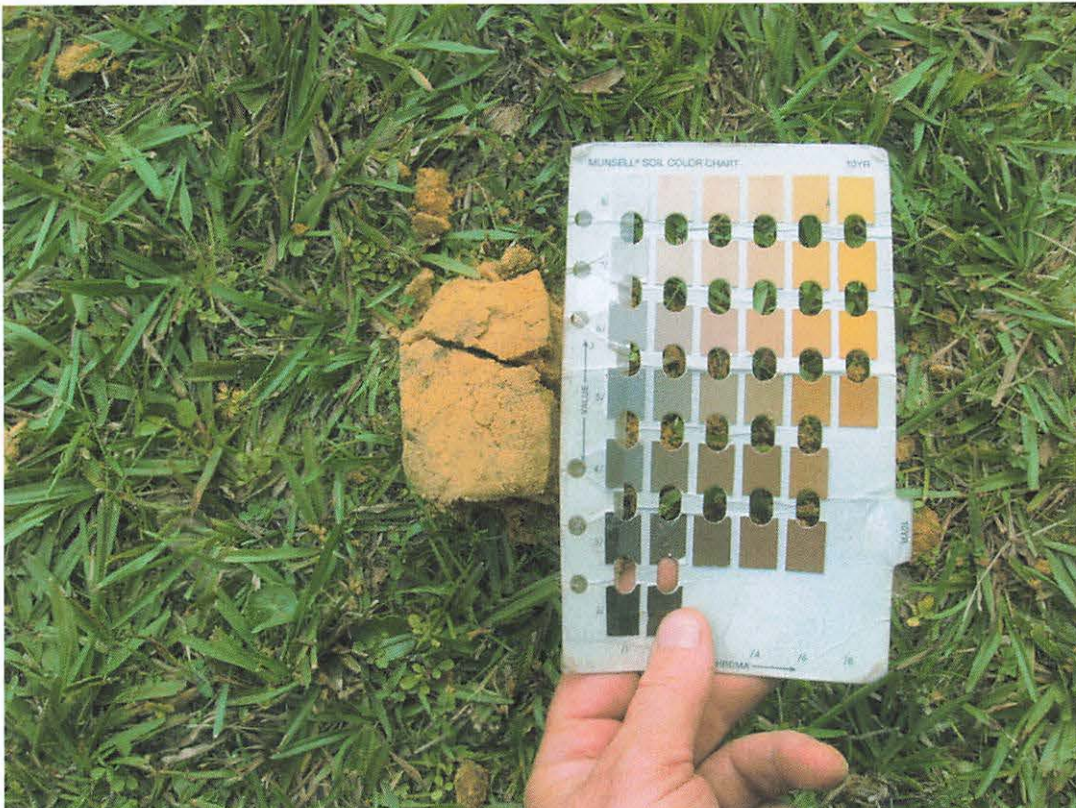
Non-hydric soil found within and indicative of Data Plot-3 (Sectional view 4.5" - 14.5" range with Munsell Soil Color Chart).
