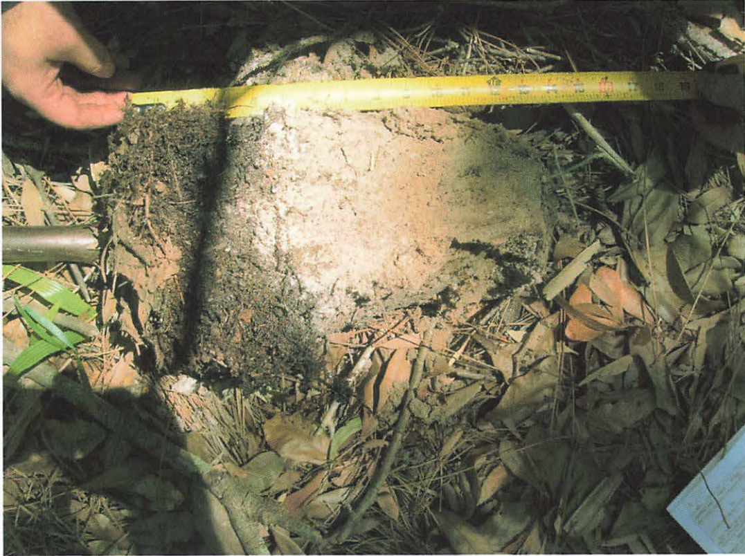
Non-hydric soil found within and indicative of Data Plot-2 (overall view with tape).
