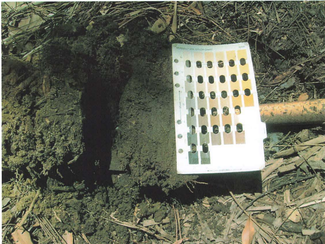
Non-hydric soil found within and indicative of Data Plot-1 (Sectional view 0" - 4.5" range with Munsell Soil Color Chart).
