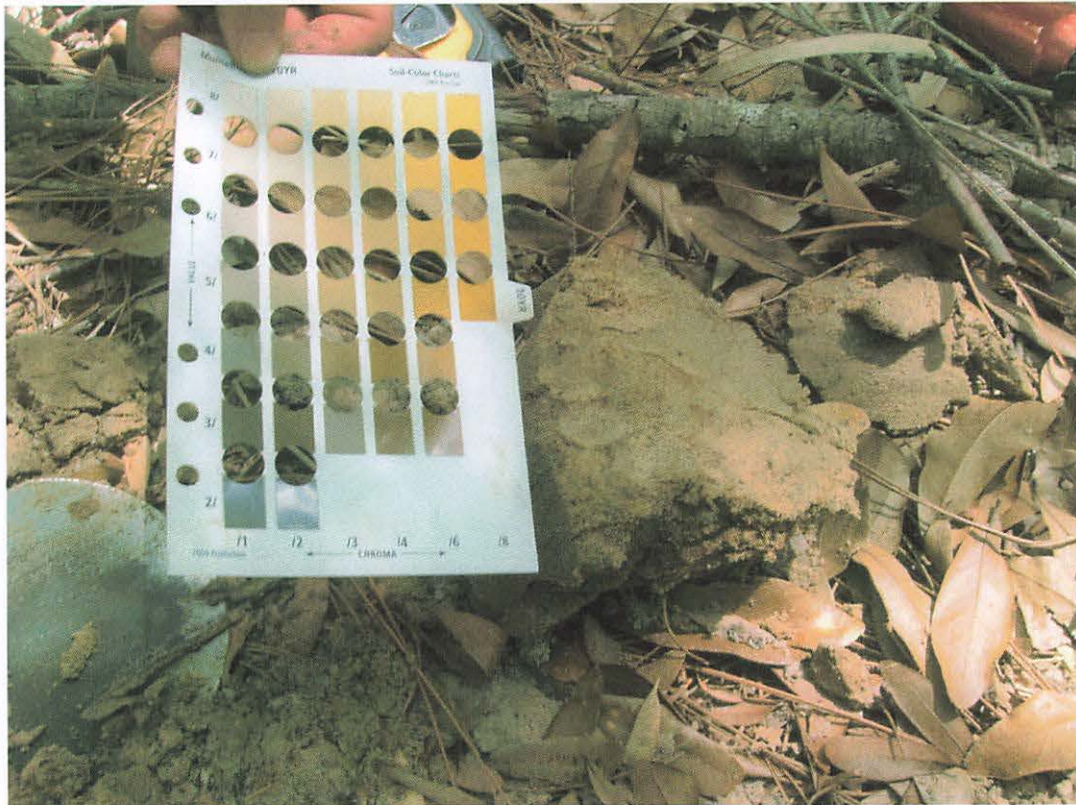
Non-hydric soil found within and indicative of Data Plot-2 (Sectional view 0" - 13.5" range with Munsell Soil Color Chart).
