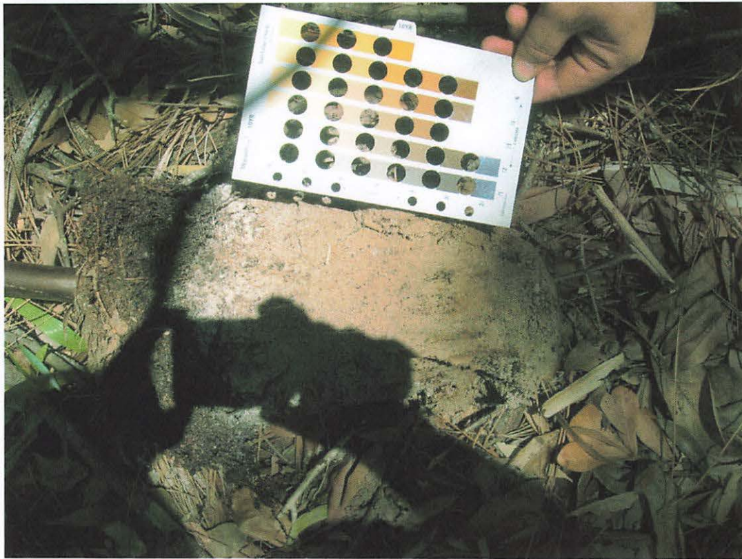
Non-hydric soil found within and indicative of Data Plot-2 (overall view with Munsell Soil Color Chart).
