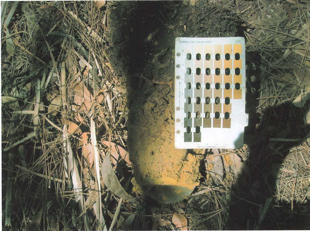
Non-hydric soil found within and indicative of Data Plot-1 (overall view with Munsell Soil Color Chart).
