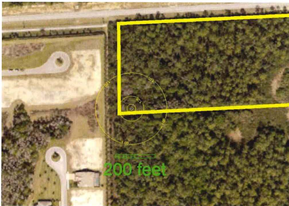
Figure 1: Drawdown Contours of Proposed Irrigation Well.
