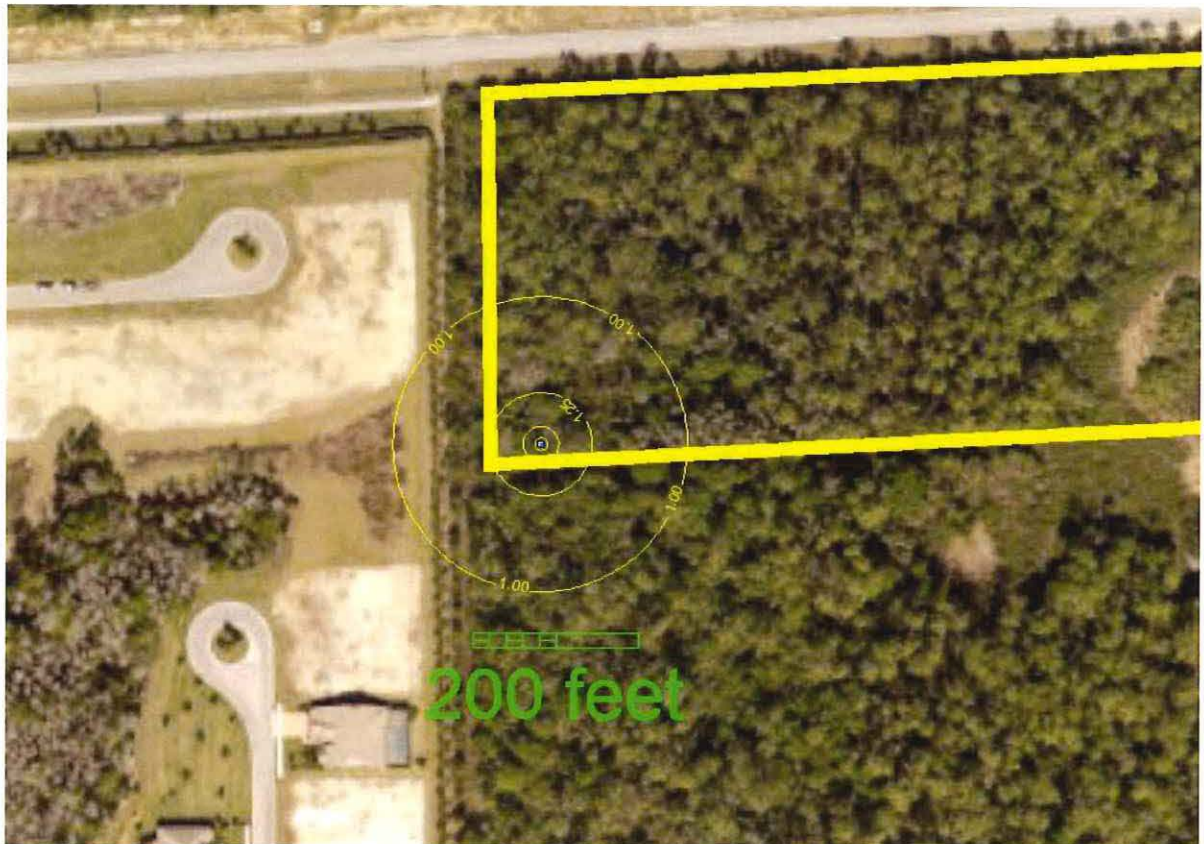
Figure 5: Drawdown Contours of Proposed Irrigation Well.
