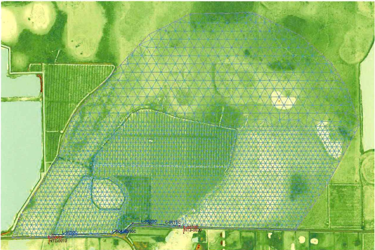
Figure II-A. 2D overland computational mesh, with LiDAR.
