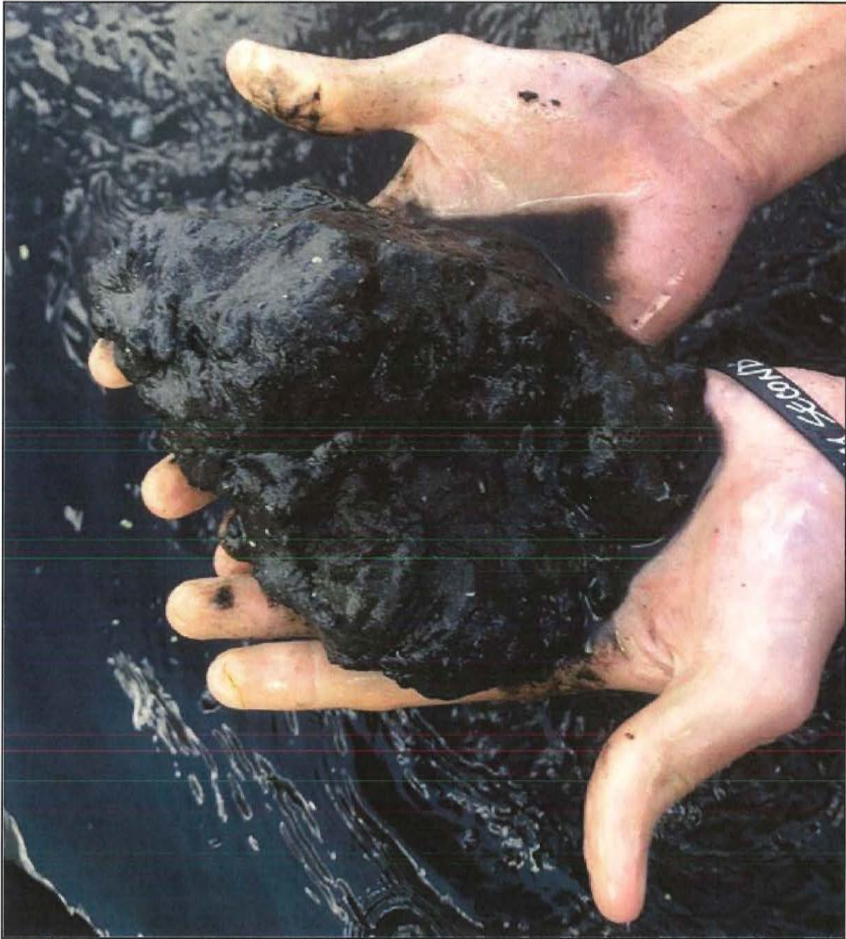
This is a typical example of the substrate that constitutes the bottom within the footprint of the propose marina basin and entrance channel. Hand grab samples were consistently the same, fine silty sand, with organics and shell fragments.
