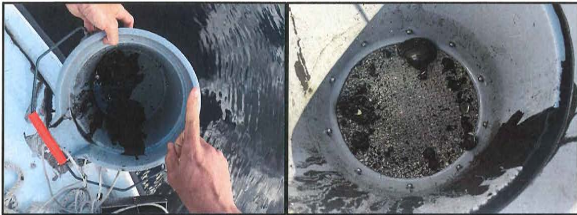
Ponar grab sample #1, on the left, and washed on the right with only shell fragments and organic debris evidenced in the substrate.
