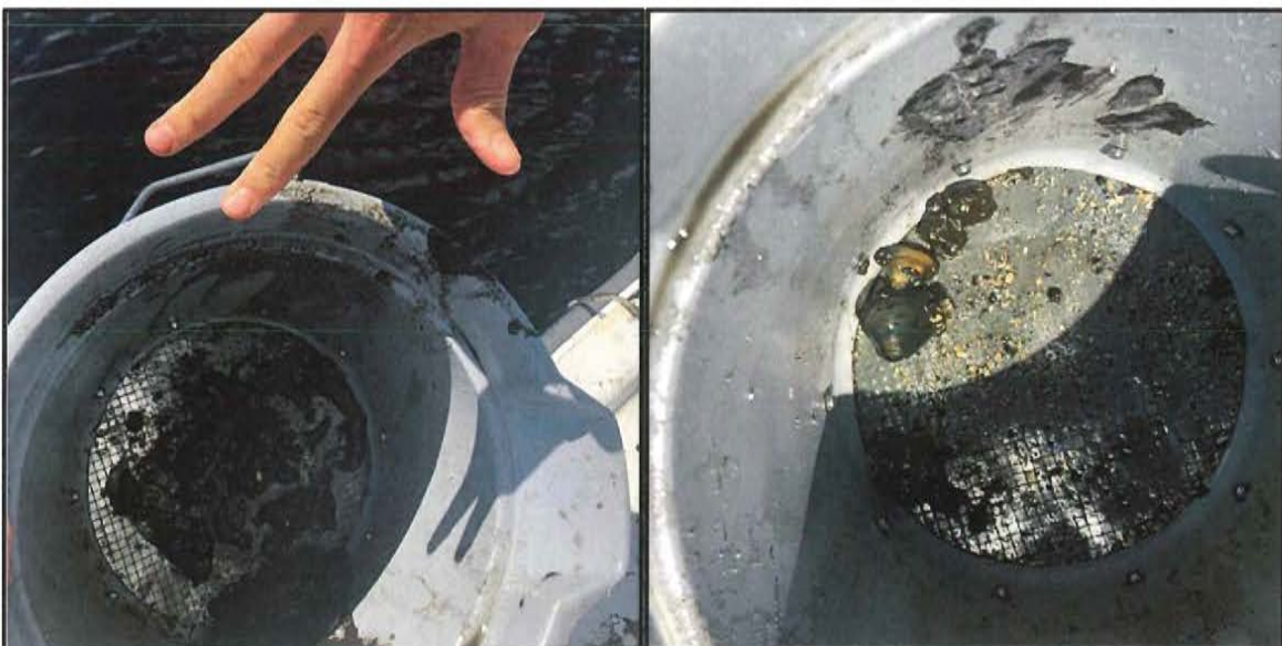
Ponar grab sample #3, on left and washed on the right. Bivalves were all dead.
