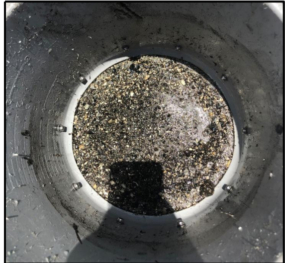
Ponar grab sample #4, black goopy muck on the left and shell fragments when washed through the sieve on the right.
