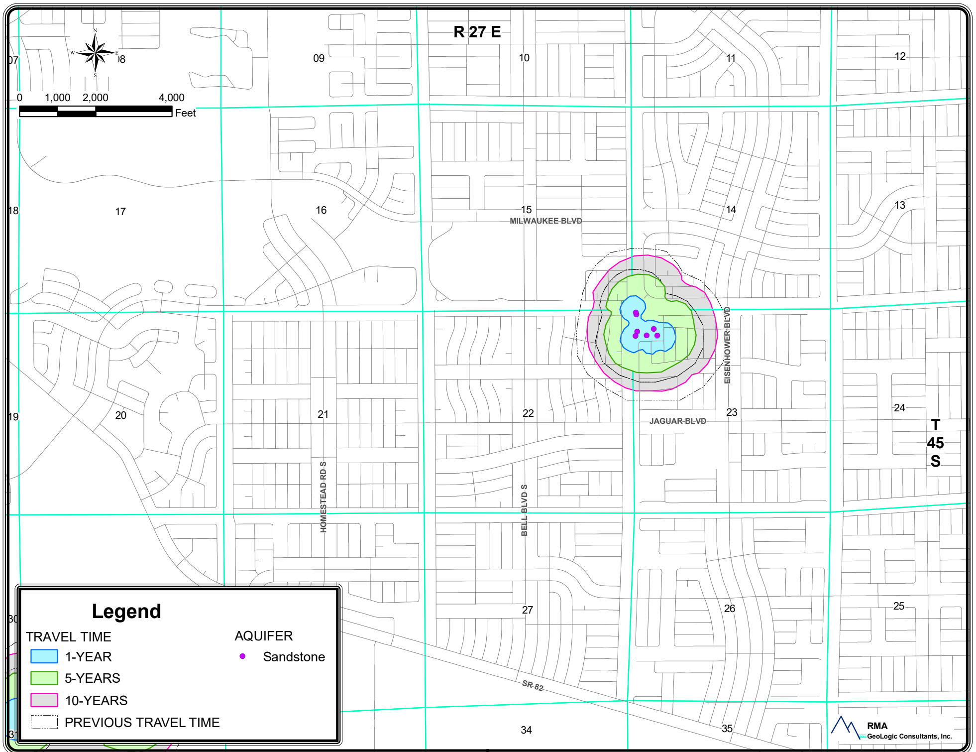
FIGURE 3-8B. MAP SHOWING PRODUCTION WELLS AND ISO-TIME CONTOURS FOR FGUA SOUTH LEHIGH WELLFIELD.
