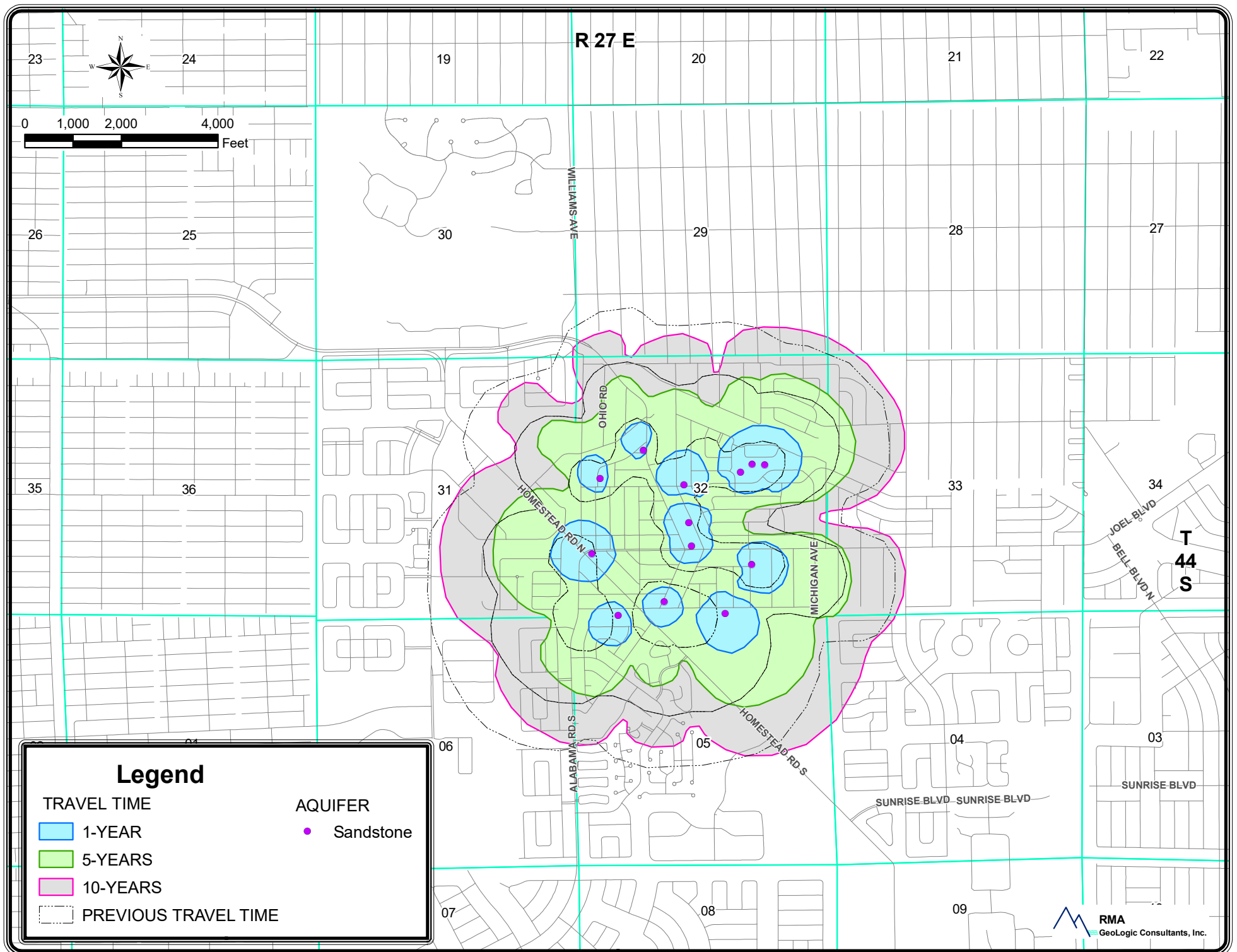
FIGURE 3-8A. MAP SHOWING PRODUCTION WELLS AND ISO-TIME CONTOURS FOR FGUA NORTH LEHIGH WELLFIELD.
