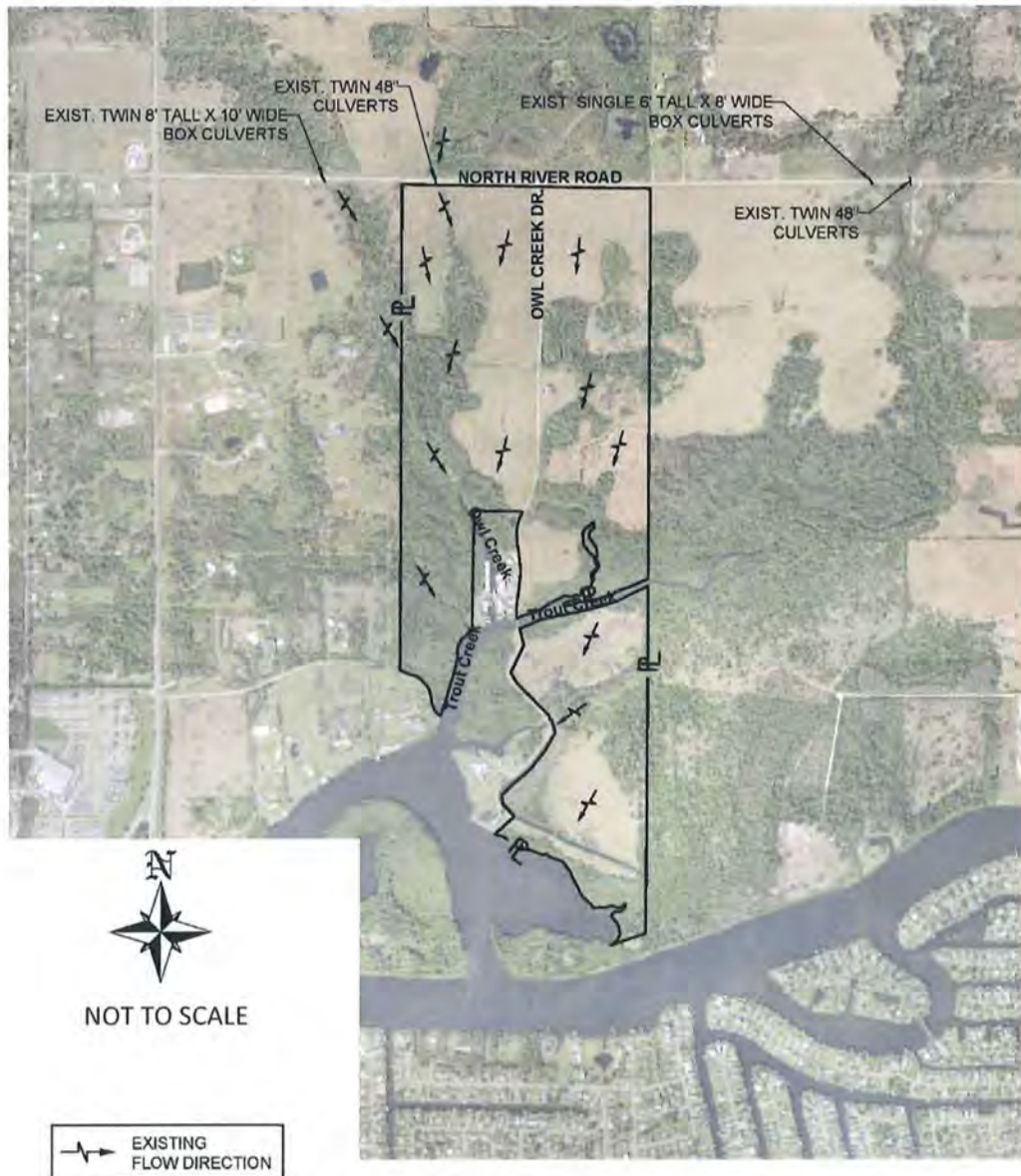
Figure 1: Existing Drainage Map
