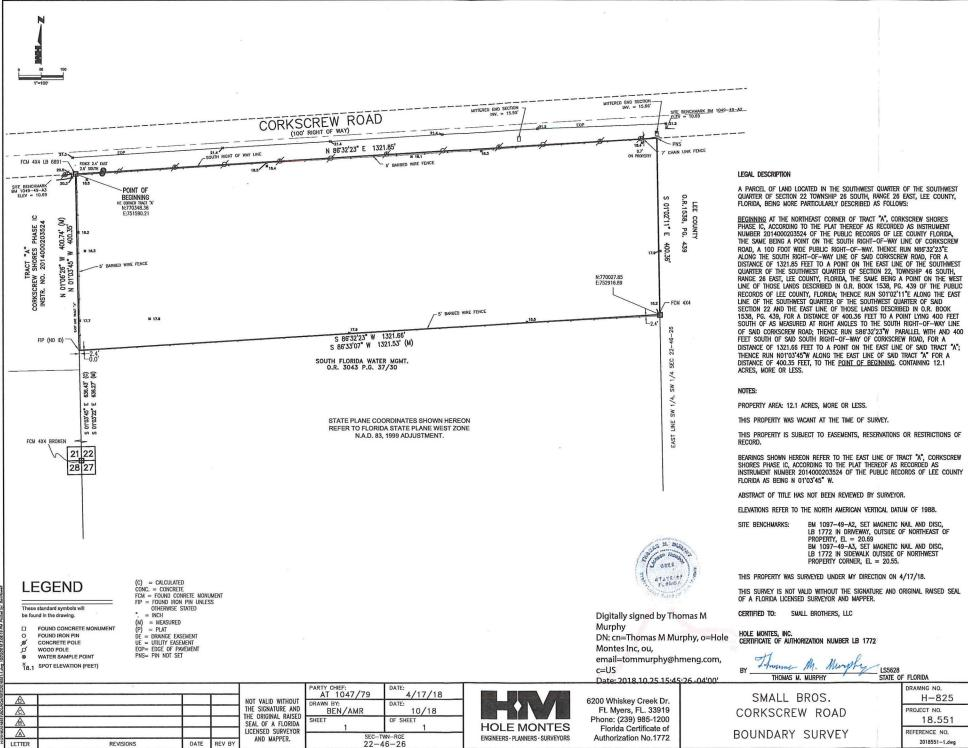
BM 1097-49-A2, SET MAGNETIC NAIL AND DISC, LB 1772 IN ORVEWAY, OUTSIDE OF NORTHEAST OF PROPERTY, EL = 20.69 BM 1097-49-A3, SET MAGNETIC NAIL AND DISC, LB 1772 IN SIDEWALK OUTSIDE OF NORTHWEST PROPERTY CORNER, EL = 20.55.
