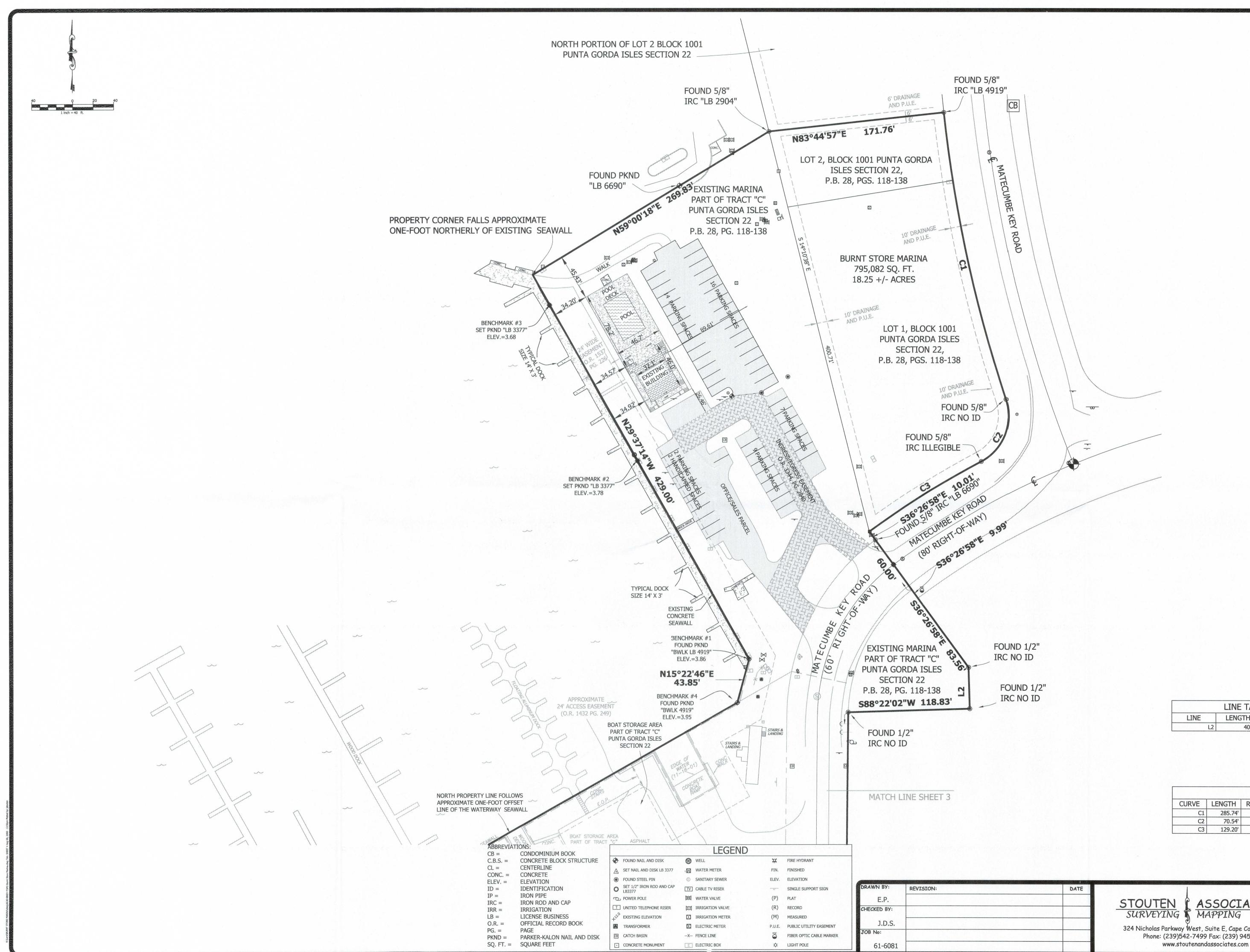
LINE TABLE LINE LENGTH BEARING 40.00 S01°37'58"E 12 CUEL AUG 1 3 2008 COMMUNITY DEVELOPMENT **CURVE TABLE** CURVE LENGTH RADIUS CH. BEARING CHORD DELTA 285.74' 1340.00' 285.20' 12°13'04" C1 S12°21'35"E S21°56'50"W 70.54' 50.00' 64.83' 80°49'54" C2 C3 129.20' 840.00' S57°57'25"W 129.07' 8°48'45" A2007-00054 STOUTEN SURVEYING MAPPING SEE SHEET 1 FOR SIGN AND SEAL 324 Nicholas Parkway West, Suite E, Cape Coral. FL 33991 SHEET 4 OF 4 Phone: (239)542-7499 Fax: (239) 945-0244
