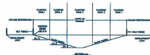
WETLAND RESTORATION CROSS-SECTION
