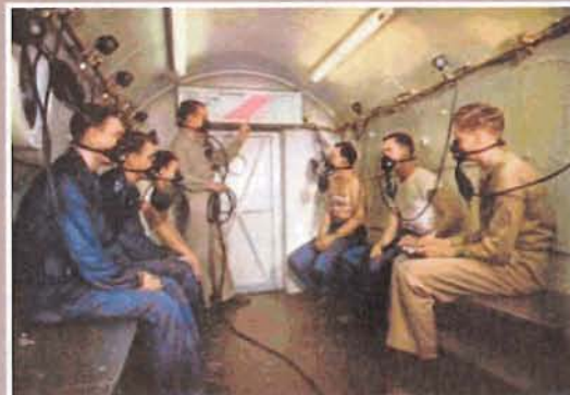
The Low Pressure Chamber took student gunners to the bombers operating altitudes without ever leaving the ground.
