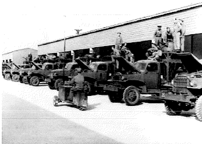
Figure 6. Gun turrets mounted to the backs of trucks, 1945 photo from the Buckingham Air Field.
