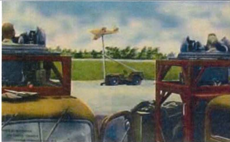
Color postcard from Tyndall Field Gunnery School shows Martin turrets mounted on trucks with an airplane mockup mounted on a jeep. The jeep is hooked to a track system.
