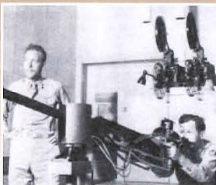
The Jam Handy trainer used images projected onto a screen. The student aimed his .50 cal. MG at the images using an optical sight.
