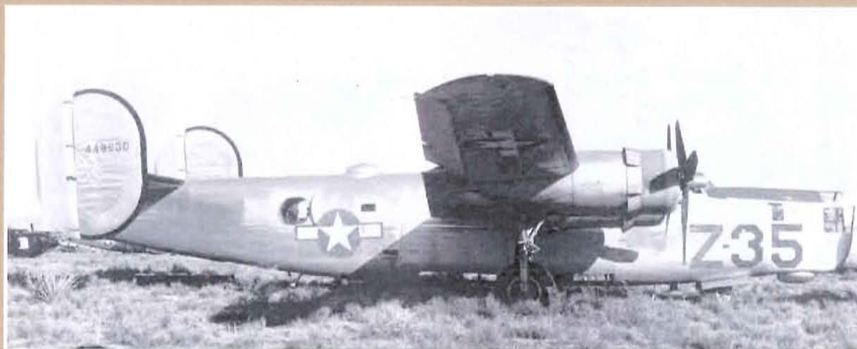
The RB-24L. One of a hand full of Liberators equipped with B-29 turrets and fire-control system and used to train gunners destined for the Superfortress.
