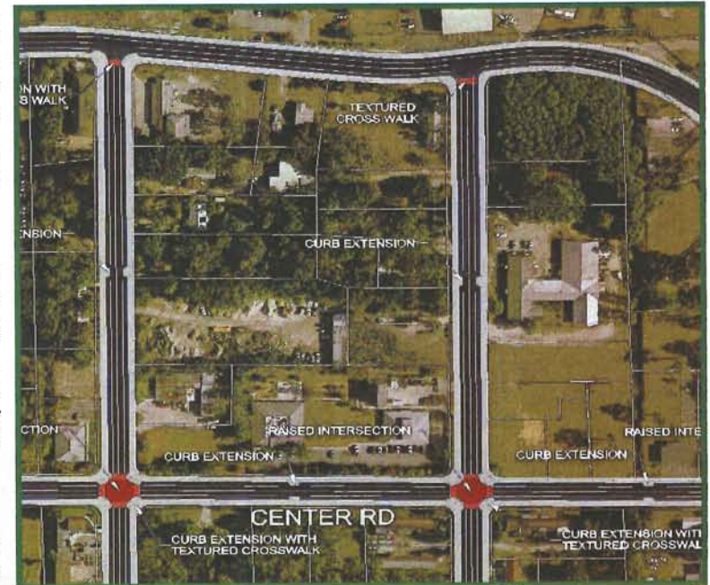
Section of traffic calming plan showing some of the techniques used such as textured crosswalks, raised intersections, and curb extensions.
