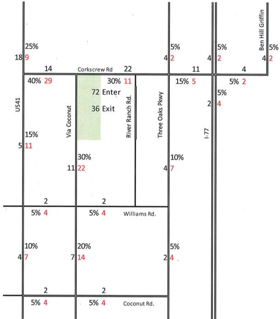
Figure 3: Project Trips Directional Distribution
