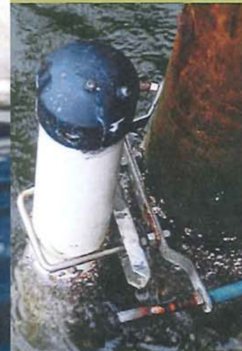
Water quality probe attached to a piling
