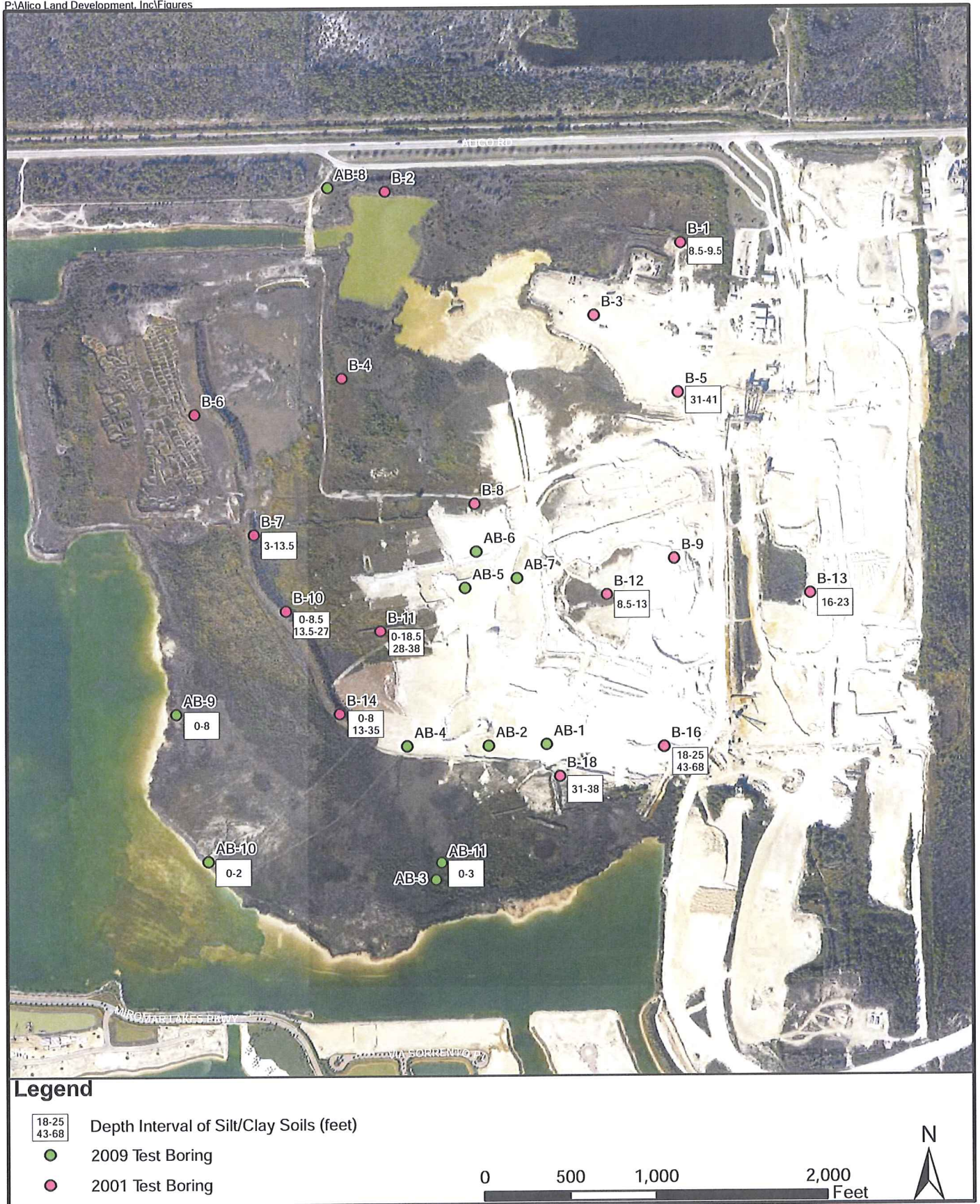
Figure 2-5 Alico Land Development, Inc. Test Borings with Thickness of Silt/Clay Soils
