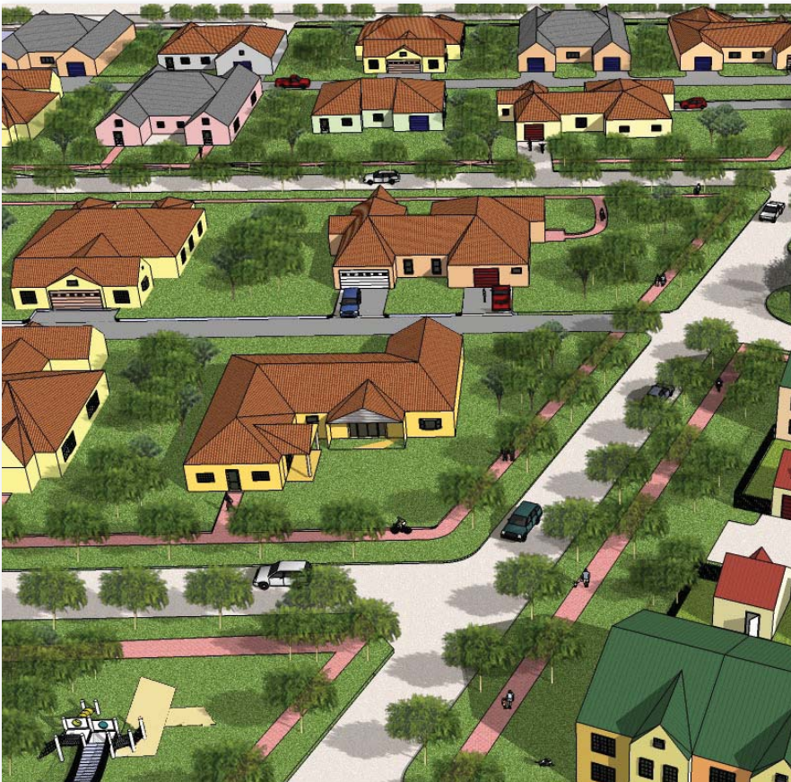
Figure 52: New prototype of duplex development with mid-block alley and rear-facing attached garages
